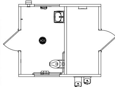
CXT buildings are delivered to your site ready to use and require minimal site preparation. Our structures are manufactured with high-strength precast concrete floors, walls, and roofs and can withstand extreme conditions caused by flood, snow, wind, and zone-4 seismic loads.
